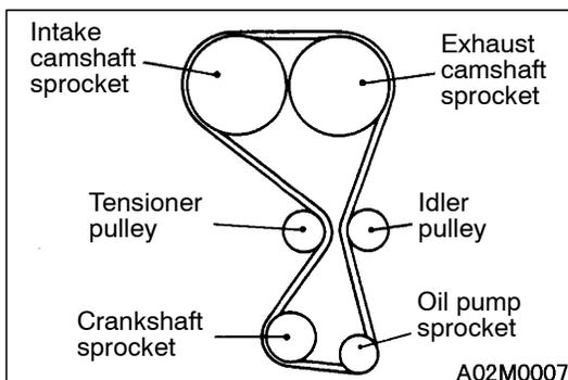
3. Position the timing belt without having any slack at the tension side of the belt.
