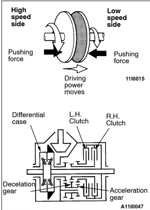
**TORQUE TRANSFER DIFFERENTIAL MECHANISM**
