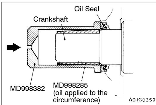
**▶◀ CRANKSHAFT FRONT OIL SEAL INSTALLATION**
