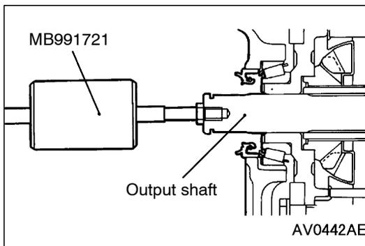
**◀C▶ OUTPUT SHAFT REMOVAL**
