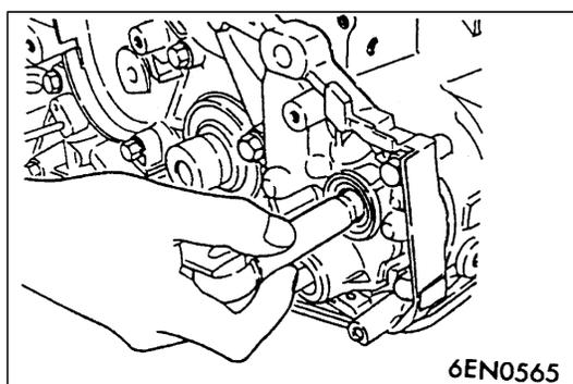
**◀D▶ COUNTER BALANCE SHAFT FRONT BEARING REMOVAL**
