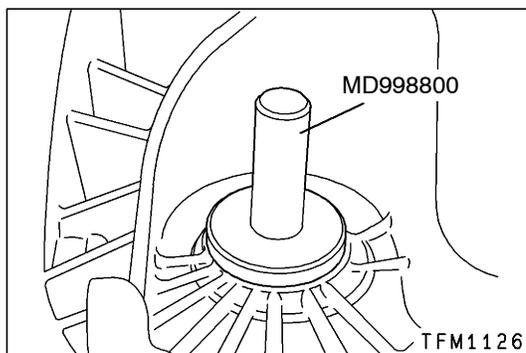
(2) Using the special tool, install the oil seal onto the transmission case.
