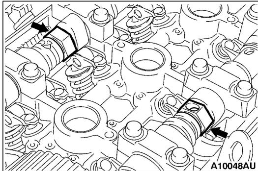
**◀B▶ CAMSHAFT SPROCKET REMOVAL**
