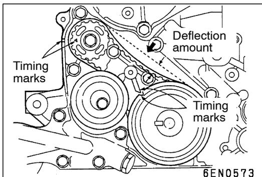
12. When measuring with the deflection amount, press the centre of the tensed side of timing belt B with your index finger in the arrow direction, and confirm that the deflection is between 5 and 7 mm.
