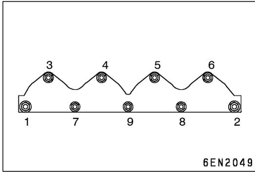
**INSTALLATION SERVICE POINTS****►A◄ EXHAUST MANIFOLD INSTALLATION**
