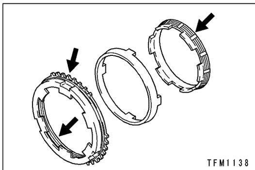
**OUTER SYNCHRONIZER RING, INNER SYNCHRONIZER RING AND SYNCHRONIZER CONE**
