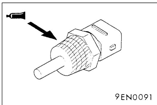
**▶D◀ ENGINE COOLANT TEMPERATURE SENSOR INSTALLATION**
