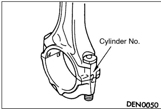
**REMOVAL SERVICE POINTS****◀A▶ CONNECTING ROD CAP REMOVAL**
