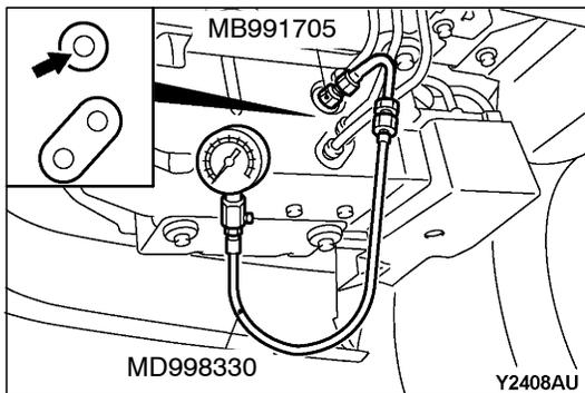
**HYDRAULIC PRESSURE CHECK <VEHICLES WITH ACD OR VEHICLES WITH ACD AND AYC>**
