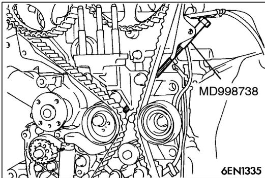
16. Set the special tool, and screw it in until the wire inserted when the auto tensioner was installed slightly moves.
