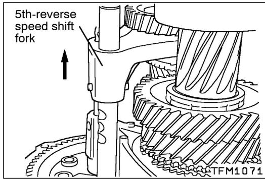
**DISASSEMBLY SERVICE POINTS****◀A▶ SPRING PIN REMOVAL**
