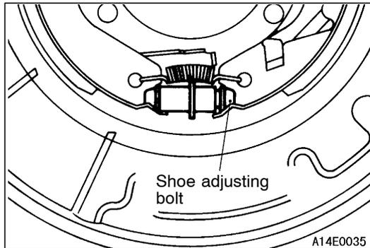
**INSTALLATION SERVICE POINTS****▶A◀ ADJUSTER ASSEMBLY INSTALLATION**
