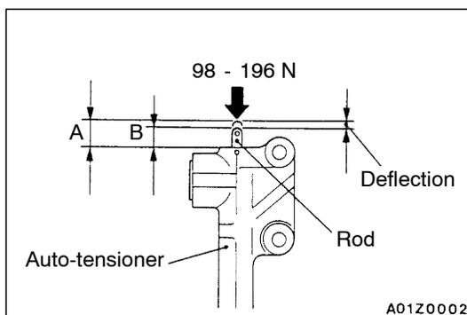
3. Measure the deflection of the rod end pressed against the metal (cylinder block, etc) with the force of 98 - 196 N while holding the auto-tensioner with a hand.
