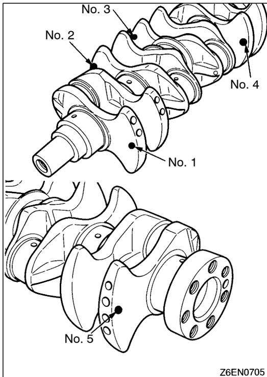
**►B◄ CRANKSHAFT BEARING INSTALLATION**
