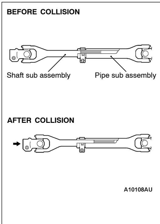
**SHOCK ABSORBING MECHANISM**
