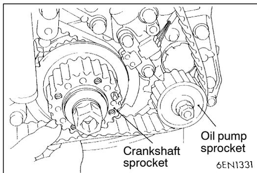
10. Attach the timing belt in the order of the idler pulley, oil pump sprocket and crankshaft sprocket.
