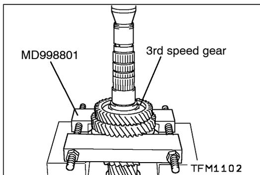
**◀D▶ 3RD SPEED GEAR REMOVAL**
