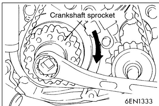
12. Rotate the crankshaft sprocket slightly in the clockwise direction, and remove the timing belt deflection on the idler pulley side.
