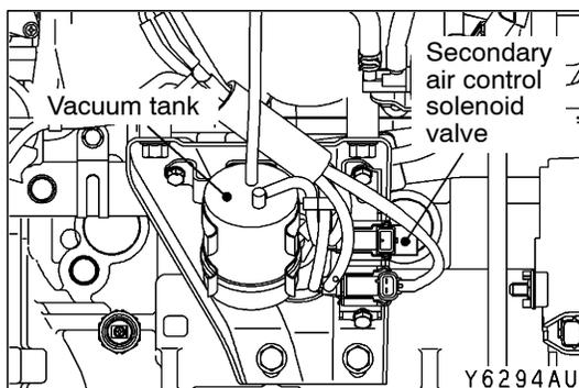
**SECONDARY AIR CONTROL SOLENOID VALVE CHECK****OPERATION CHECK**
