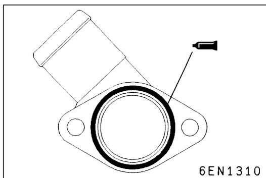
**▶B◀ WATER OUTLET FITTING INSTALLATION**
