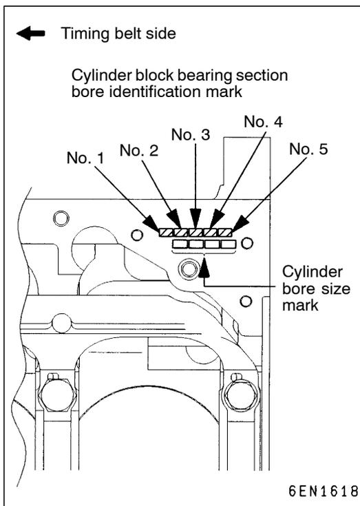
2. The cylinder block bearing section bore identification mark is stamped at the position shown in the illustration.
