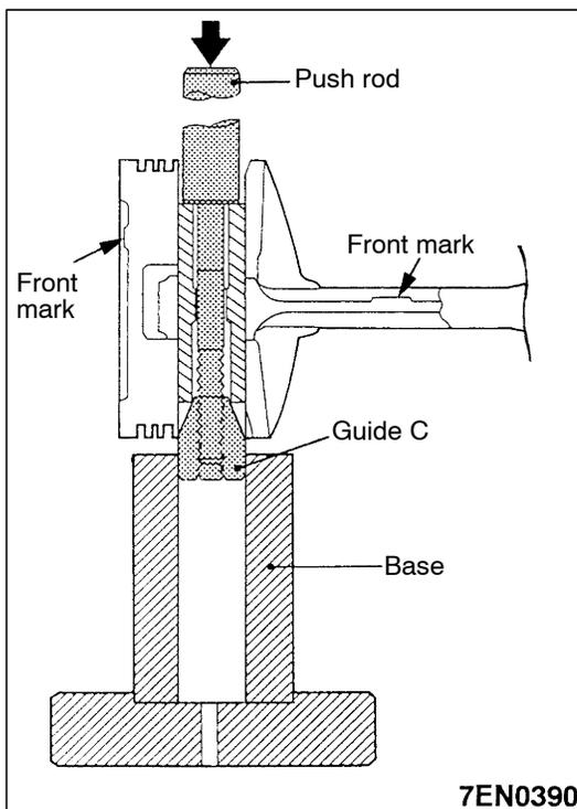
1. Insert the special tool's push rod in from the front mark (arrow) side of the piston's front face, and install guide C.
