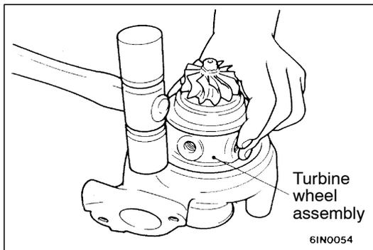
**◀B▶ TURBINE WHEEL ASSEMBLY REMOVAL**
