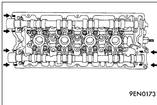
3. Apply sealant on the contact surfaces with the head shown in the illustration.
