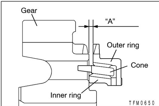
(2) Assemble the outer ring, inner ring and cone. Press against the gears and check the clearance "A". Replace if "A" is less than the limit value.
