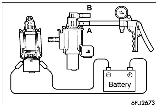
3. Connect the hand vacuum pump to the solenoid valve's A nipple.
