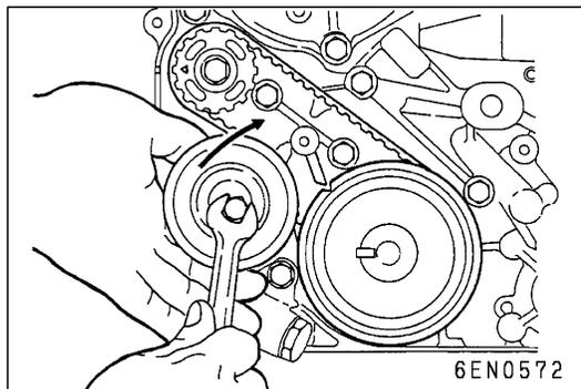
3. Confirm that the tensioner B centre and bolt centre are positioned as shown in the illustration.
