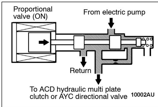
When the proportional valve turns ON, the proportional valve opens, and the oil pressure from the electric pump will be supplied to the ACD hydraulic multi plate clutch or AYC directional valve.
