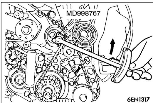
17. Loosen the tensioner pulley fixing bolt.
