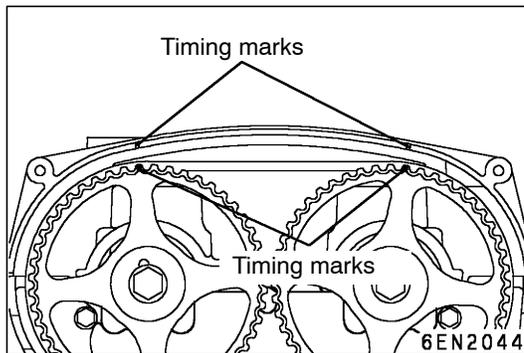
9. Rotate the exhaust side camshaft sprocket in the clockwise direction, and confirm that the intake side camshaft sprocket's timing marks are aligned when the timing marks are aligned.
