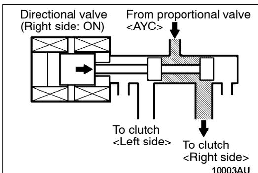
When oil pressure supply signal for the AYC clutch <Right side> is sent to the directional valve from the 4WD-ECU, the directional valve will move to the right. As a result, the oil pressure from the proportional valve <AYC> will be supplied to the AYC clutch <Right side>.
