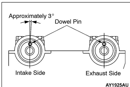
**▶C◀ CAMSHAFT BEARING CAP NO.4/CAMSHAFT BEARING CAP NO.3/CAMSHAFT BEARING CAP NO.5/CAMSHAFT BEARING CAP NO.2/CAMSHAFT BEARING CAP REAR/CAMSHAFT BEARING CAP FRONT INSTALLATION**
