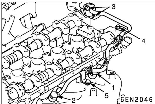
**▶D◀ AIR PIPE ASSEMBLY INSTALLATION**
