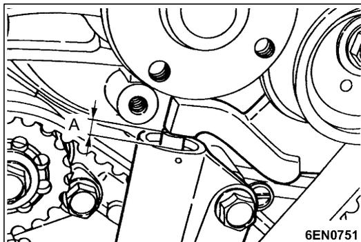
6. Remove a wire or a pin inserted during installation of the automatic tensioner.
