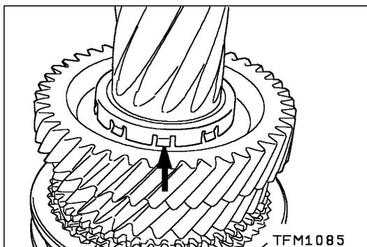
**◀B▶ THRUST PLATE STOPPER REMOVAL**
