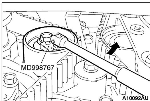
4. Use the special tool to rotate the tensioner pulley in the direction indicated in the figure, tighten the timing belt, and temporarily tighten the mounting bolt of the tensioner pulley for fixing.
