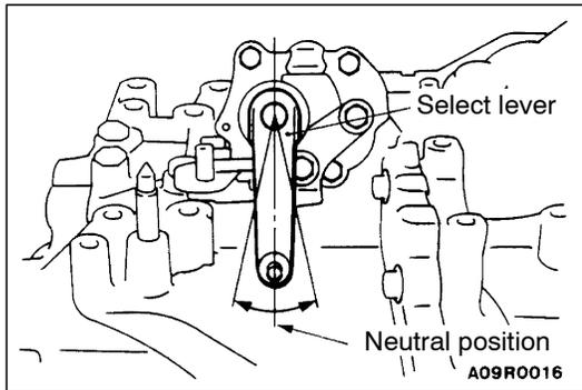
**INSTALLATION SERVICE POINT****▶A◀ CLIP/SELECT CABLE AND SHIFT CABLE ASSEMBLY/SHIFT CABLE CONNECTION/SELECT CABLE CONNECTION INSTALLATION**
