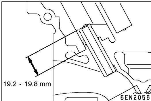
3. Press in the valve guide to the dimensions shown in the illustration.
