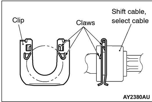
**REMOVAL SERVICE POINT****◀A▶ CLIP/SELECT CABLE CONNECTION (TRANSMISSION)/SHIFT CABLE (TRANSMISSION) INSTALLATION**
