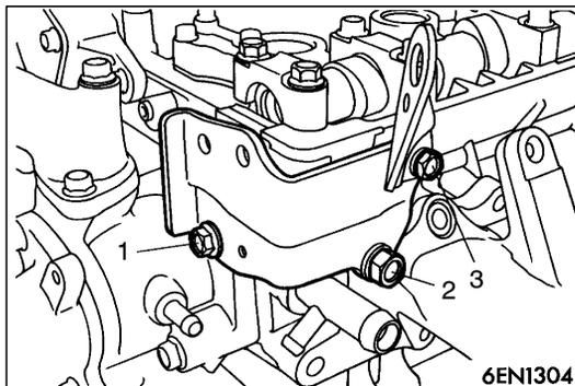
**▶C◀ AIR CONTROL VALVE BRACKET INSTALLATION**
