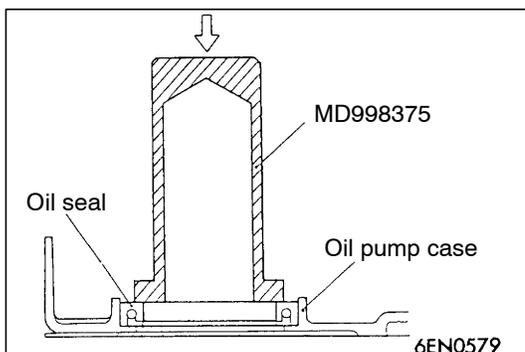
►F◄ CRANKSHAFT FRONT OIL SEAL INSTALLATION
