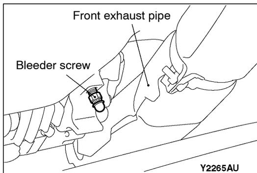
6. Remove the cap of the bleeder screw on the transfer, and connect the vinyl hose.
