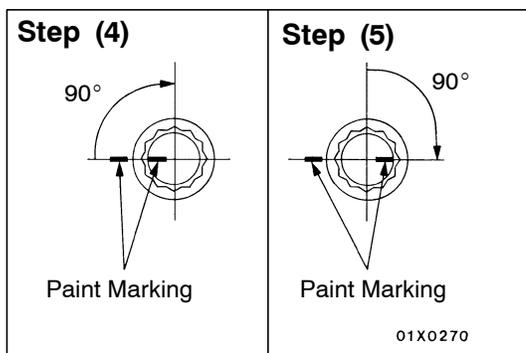
3. Use special tool to tighten bolts according to the following procedure (tightening for plastic zone)
