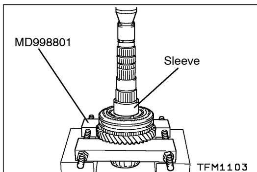
**◀E▶ 2ND SPEED GEAR SLEEVE REMOVAL**
