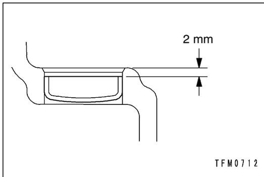
**▶C◀ SEALING CAP INSTALLATION**
