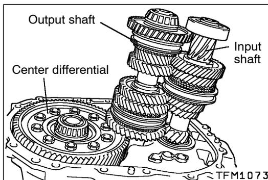
**ADJUSTMENT BEFORE REASSEMBLY****SELECTION OF INPUT SHAFT END PLAY/OUTPUT SHAFT END PLAY/OUTPUT SHAFT PRELOAD AND CENTER DIFFERENTIAL PRELOAD ADJUSTMENT SPACER**
