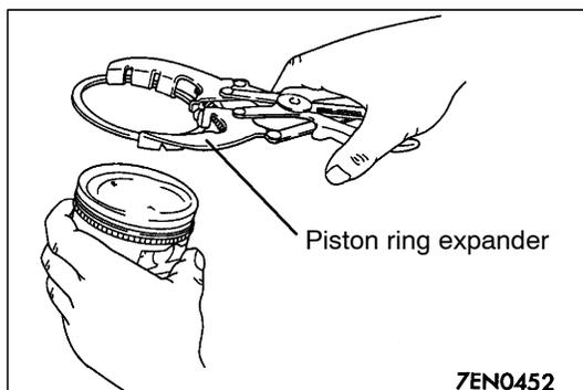
►C◄ PISTON RING NO. 2/PISTON RING NO. 1 INSTALLATION
