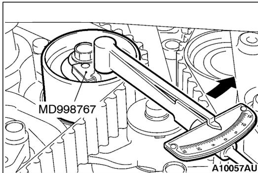
5. Use the special tool and torque wrench to apply tension torque (3.5 N·m) to the timing belt in the direction indicated in the figure and tighten the tensioner pulley mounting bolt to the specified torque.
