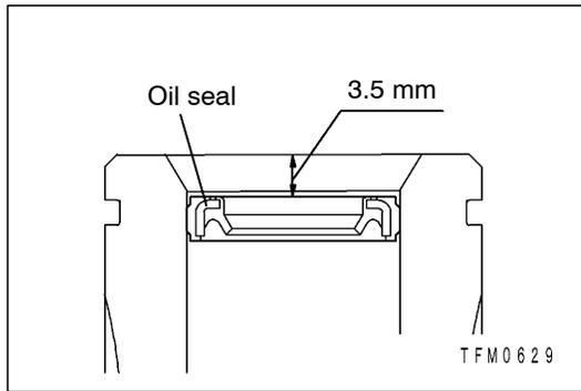
**REASSEMBLY SERVICE POINTS****▶A◀ OIL SEAL INSTALLATION**
