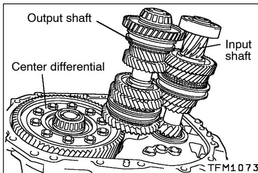
**◀C▶ CENTER DIFFERENTIAL/OUTPUT SHAFT/INPUT SHAFT REMOVAL**
