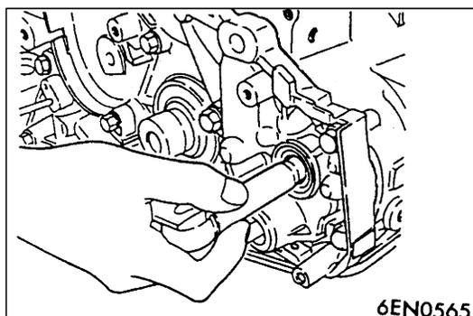
2. Tighten the flange bolt at the specified torque  $36 \pm 3 \text{ N}\cdot\text{m}$ .
