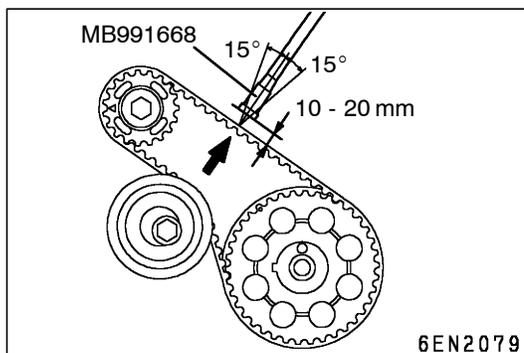
9. Separate the special tool (MB991668) 10 to 20 mm from the centre back between the sprockets (shown with an arrow), and hold so that it is vertical (inclination within  $\pm 15^\circ$ ) in respect to the belt.
