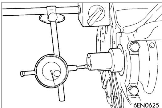
8. After installing the beam bearing cap, inspect the end play of the crankshaft. If the end play exceeds the limit value, replace the crankshaft bearing.
