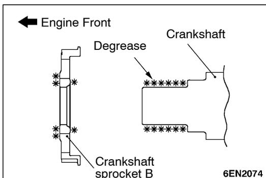
**▶◀ CRANKSHAFT SPROCKET B INSTALLATION**
