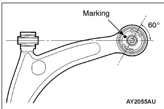
2. Set the bushing to the lower arm assembly in order to the direction of bushing marking is upper, and of the opening is the direction as shown in the illustration.
