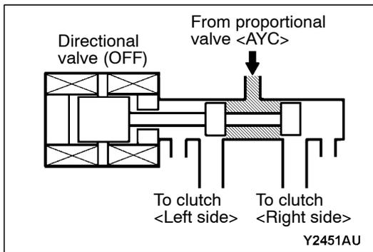
When the directional valve is OFF, the oil pressure from the proportional valve <AYC> will be cut off by the directional valve. For this reason, the clutch will set into the non-operating state without oil pressure supplied to each clutch of the AYC.
