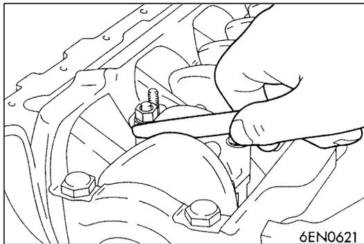
9. Check that the thrust clearance at the large end of the connecting rod is correct.
