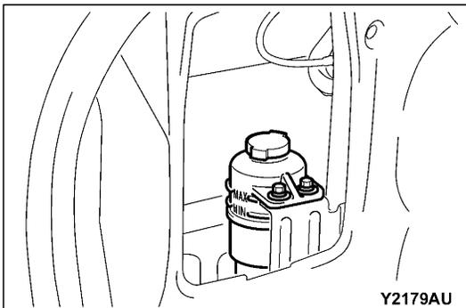
3. Check that the fluid level in the oil reservoir is in the range between MAX and MIN.
