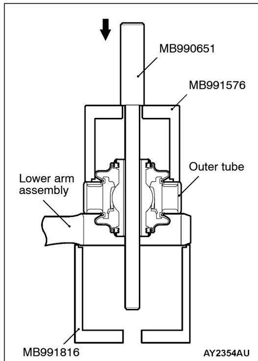
3. Use the special tools to press in the bushing until its outer tube is flush with the lower arm assembly surface.
