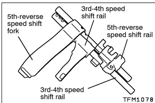
**▶B◀ 5TH-REVERSE SPEED SHIFT FORK/5TH-REVERSE SPEED SHIFT RAIL/3RD-4TH SPEED SHIFT FORK/3RD-4TH SPEED SHIFT RAIL INSTALLATION**
