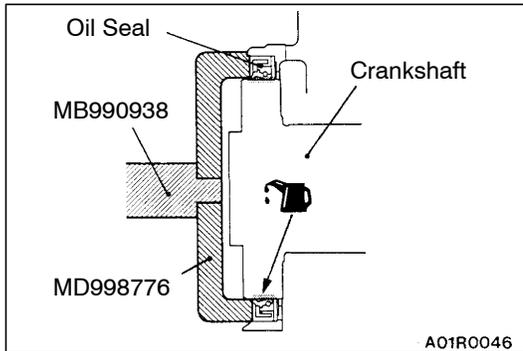
**INSTALLATION SERVICE POINTS****▶◀ CRANKSHAFT REAR OIL SEAL INSTALLATION**
