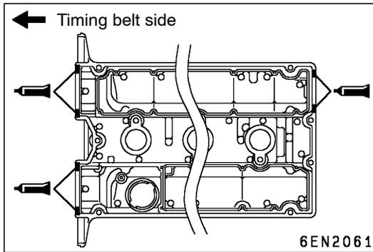
3. Apply form-in-place gasket on the rocker cover at the position shown in the illustration.
