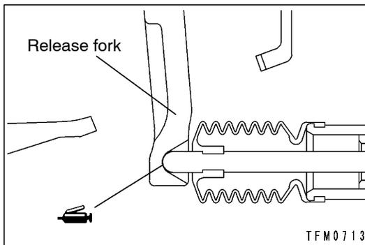
**▶D◀ CLUTCH RELEASE CYLINDER INSTALLATION**
