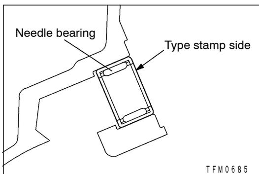
**►B◄ NEEDLE BEARING INSTALLATION**
