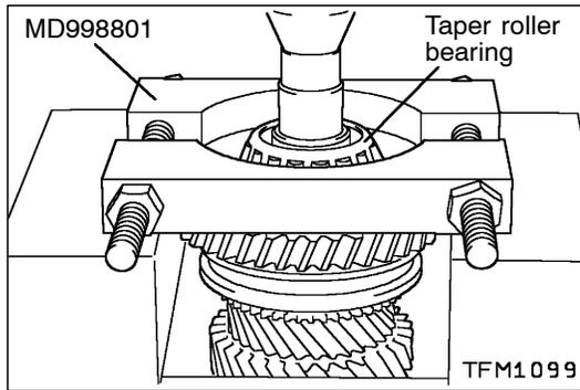
**DISASSEMBLY SERVICE POINTS****◀A▶ TAPER ROLLER BEARING REMOVAL**
