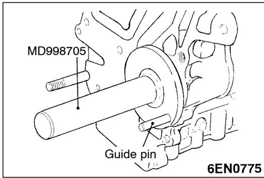
4. Align and insert the special tool into the guide pin, and tap in the counter balance shaft front bearing.
