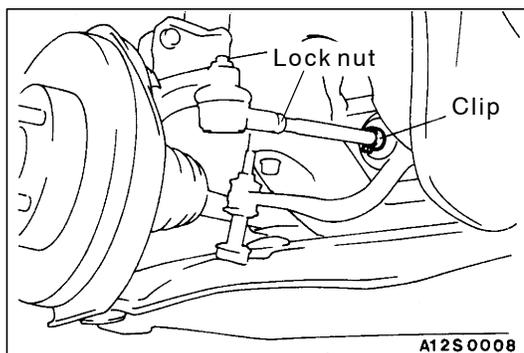
**Tightening torque:  $52 \pm 2$  N·m**
