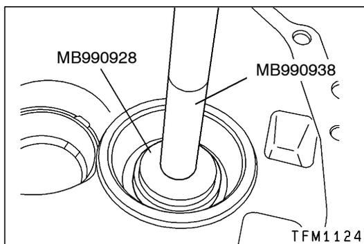
(2) Using the special tool, install the oil seal onto the clutch housing.
