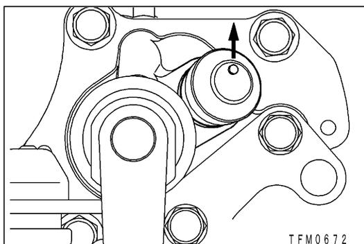
(2) Install so that the protrusion faces the direction shown in the illustration.
