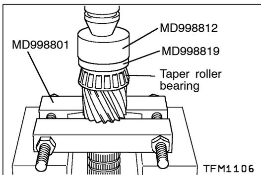
▶B◀ TAPER ROLLER BEARING INSTALLATION
