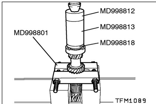
**▶B◀ BALL BEARING INSTALLATION**
