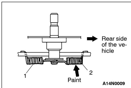
**▶B◀ SHOE-TO-ANCHOR SPRING INSTALLATION**
