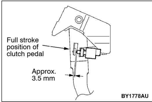
5. Fix the clutch pedal position switch by rotating approx. quarter turn to clockwise in the position as shown in the illustration.
