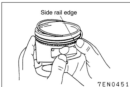
2. The side rail can be assembled easily by fitting one end of the side rail into the piston groove and then pressing on it with fingers as shown in the illustration.
