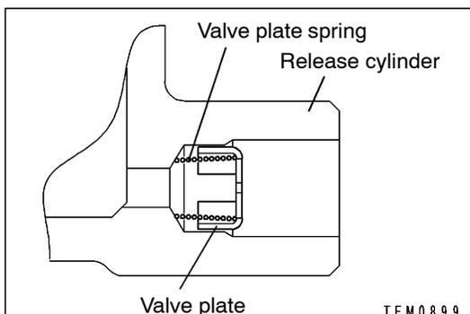
**▶E◀ VALVE PLATE SPRING/VALVE PLATE INSTALLATION**
