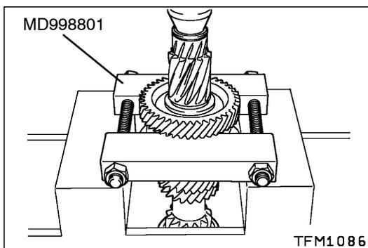
**◀C▶ 5TH SPEED GEAR REMOVAL**
