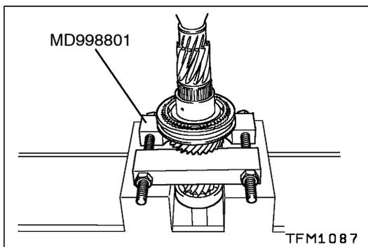
**◀D▶ 4TH SPEED GEAR SLEEVE REMOVAL**
