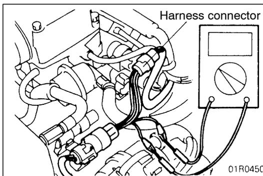
**IF INSPECTING WITH THE CONNECTOR CONNECTED (WITH CIRCUIT IN A CONDITION OF CONTINUITY)**
