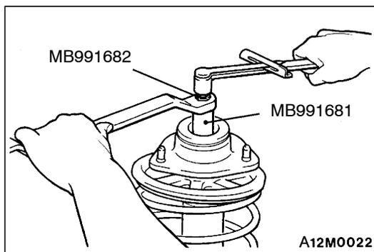
6. Using the special tools, tighten the self-locking nut to the specified torque.
