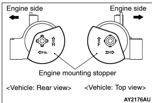
**▶B◀ ENGINE MOUNTING BRACKET AND STOPPER ASSEMBLY INSTALLATION**
