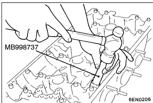
**INSTALLATION SERVICE POINTS****▶A◀ VALVE STEM SEAL INSTALLATION**
