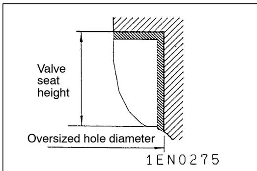
3. When pressing in the valve seat, cool the valve seat with liquid nitrogen, and make sure that the inner diameter of the cylinder head is not galled.
