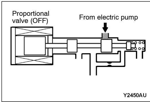
When the proportional valve is OFF, the oil pressure from the electric pump will be cut off by the proportional valve. For this reason, oil pressure will be supplied to the ACD or AYC and each system will be set into the non-operating state.
