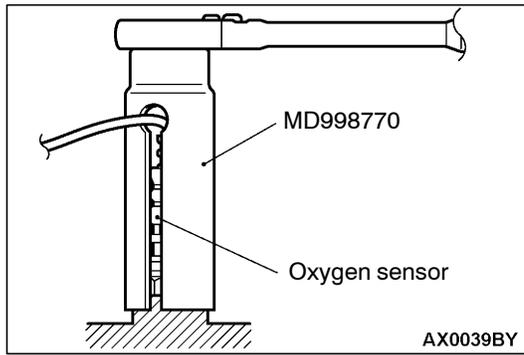
**REMOVAL SERVICE POINT****◀A▶ OXYGEN SENSOR REMOVAL**
