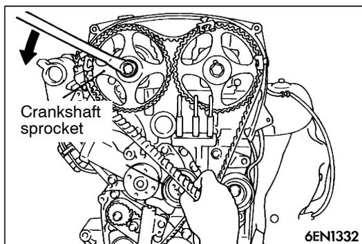
11. Attach the timing belt to the tensioner pulley.
