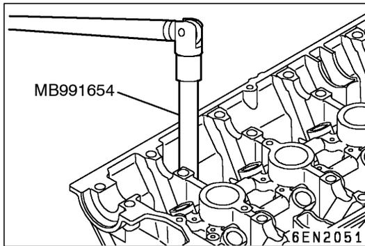
**REMOVAL SERVICE POINTS****◀A▶ CYLINDER HEAD BOLT REMOVAL**
