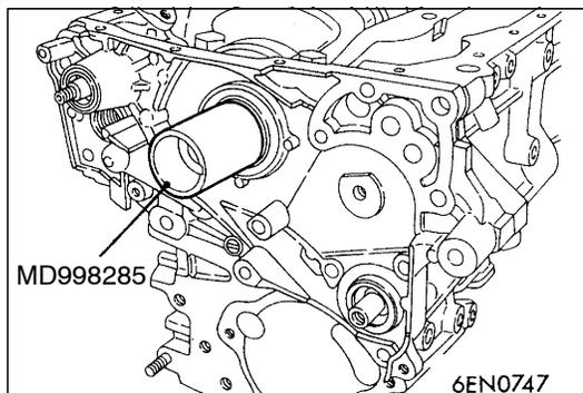
2. Install the oil pump case through the new oil pump case gasket, and temporarily tighten the bolts other than the oil filter bracket tightening bolt.
