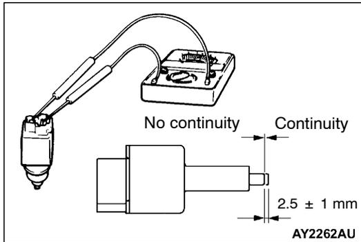
**INSPECTION****CLUTCH PEDAL POSITION SWITCH CONTINUITY CHECK**
