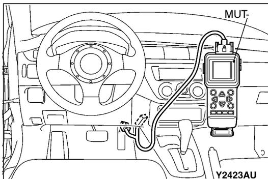
**INPUT SIGNAL CHECK <SWS>****WHEN USING THE MUT-II**
