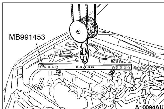
3. Hold the engine assembly with a chain block.
