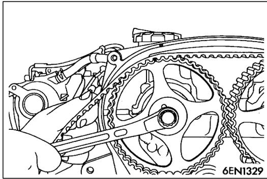
8. Rotate the intake side camshaft sprocket in the counterclockwise direction. Attach the belt at a position where the timing mark is deviated by one tooth in the counterclockwise direction, and then fix with a paper clip.
