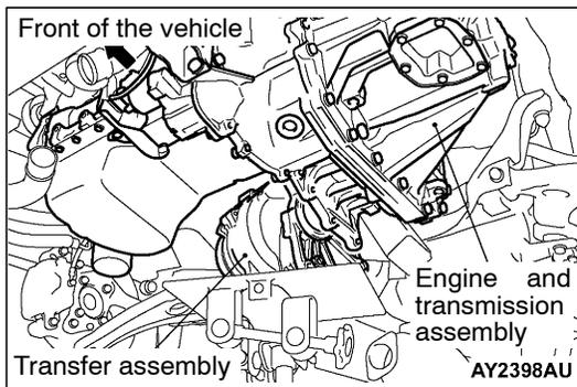
**◀D▶ TRANSFER ASSEMBLY REMOVAL**
