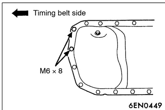
3. Note that the lengths of the bolts shown in the illustration differ, so take care when installing.
