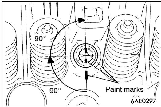
3. Following the tightening order, tighten at  $78 \pm 2 \text{ N}\cdot\text{m}$ .
