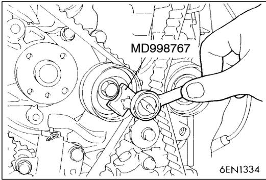
14. Using the special tool, rotate the tensioner pulley in the counterclockwise direction to tense the timing belt, and then fix by temporarily tightening the tensioner fixing bolt.
