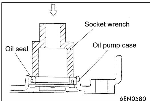
►E◄ COUNTER BALANCE SHAFT OIL SEAL INSTALLATION
