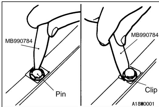
**DISASSEMBLY SERVICE POINT****◀A▶ CLIP REMOVAL**
